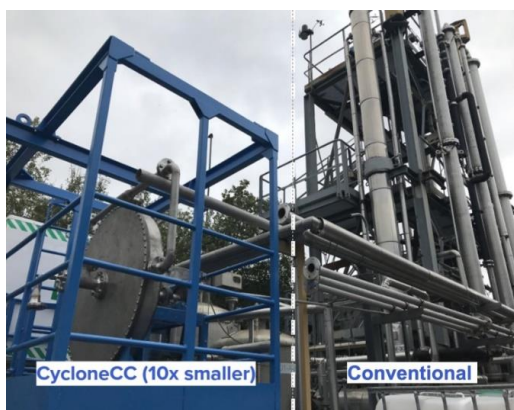
Figure 11. Reduced size of CycloneCC in comparison to the conventional capturing unit
