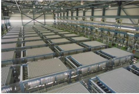
Figure 5. Chlor-alkali cell line with membrane cells 15
